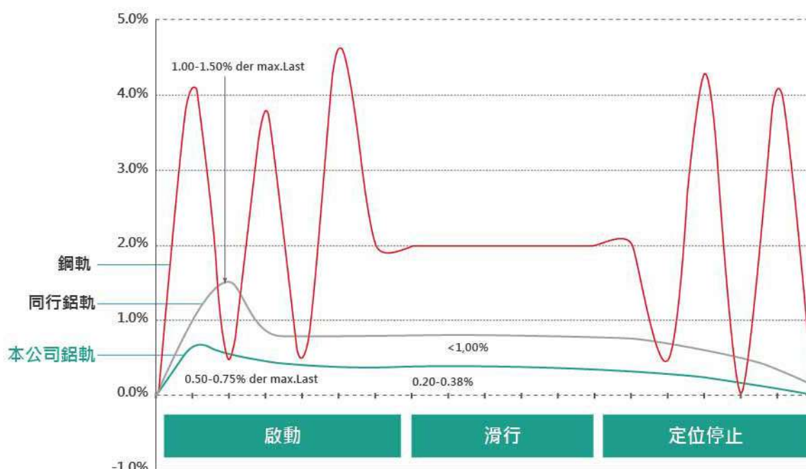
滑車運行時所需推力 / Force required when working with suspended runway systems
